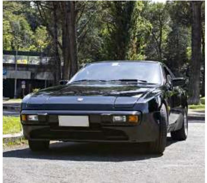
*The Porsche 944 was born as an evolution of the 924 on the price list since 1976. Based on the aesthetics of the special version called 924 Carrera GT, Harm Lagaai, the historic Porsche designer, widened the fenders, modernized the body and fitted a new 4-cylinder 2.5 liter in-line engine derived from the powerful 8-cylinder of the 928: the 944 is born and we are in 1982. The new 2479 cc engine is capable of delivering 163 HP which pushes the 944 to a top speed of 220 km/h.*
